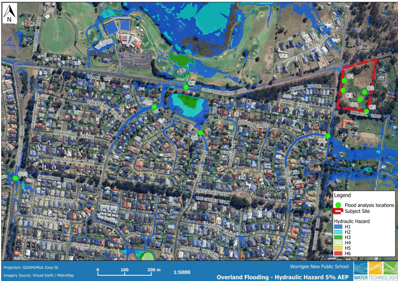
Figure 2.8 Overland flooding - Hydraulic Hazard during a 5% AEP event
