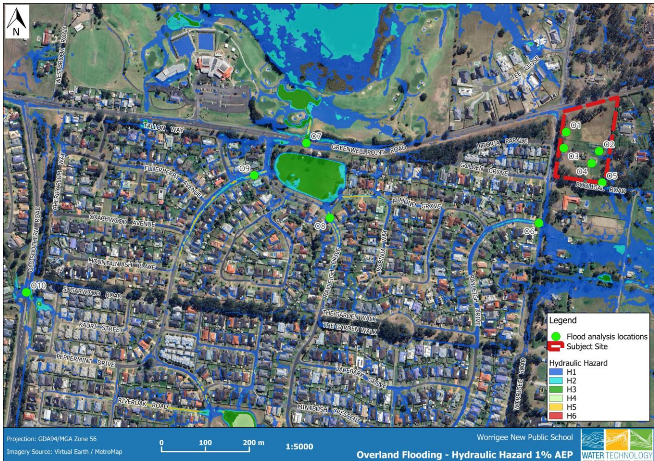
Figure 2.9 Overland flooding - Hydraulic Hazard during a 1% AEP event
