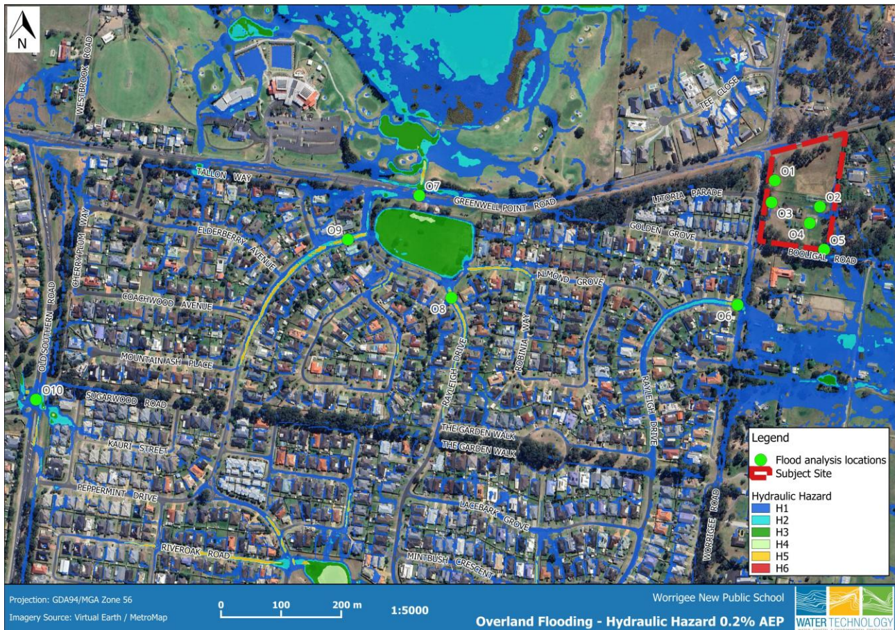
Figure 2.10 Overland flooding - Hydraulic Hazard during a 0.2% AEP event
